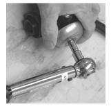
4. Check the bell to ensure that it is tight. You must not be able to rotate or tilt the bell by hand.
