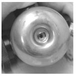
2. Using an inch pound torque wrench and a 5/16 standard 6-point socket, thread the new screw into the alarm housing.
